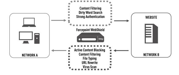
Figure 2: Forcepoint WebShield Security Controls
